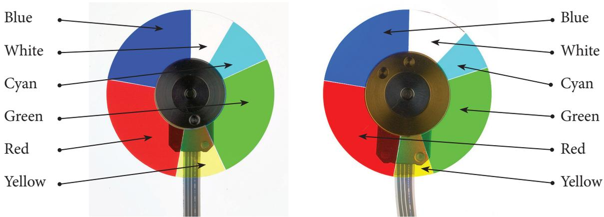
*Figure 8: 1-Chip DLP projector color wheels are photographed to show the unnecessary addition of cyan and yellow colors plus the white segment. The white segment can vary in size, directly influencing the White Light Output. Left color wheel is from InFocus IN35 1-Chip DLP projector, right color wheel is from Optoma EP728 1-Chip DLP projector.*
