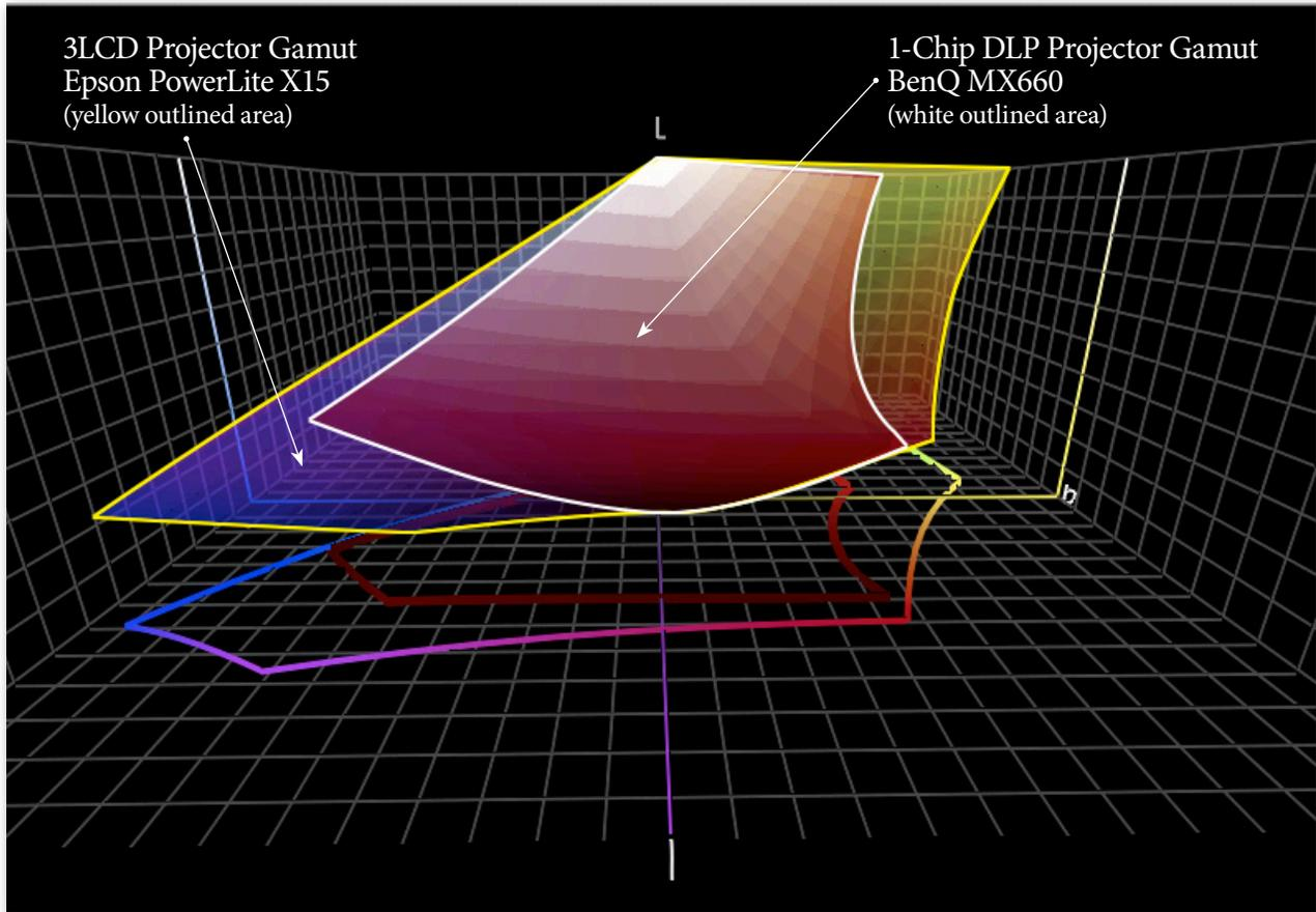
*Figure 10:* Standard color management tools were used to evaluate the gamut of a 3LCD and 1-Chip DLP projector. In this  $L^*a^*b^*$  diagram we clearly see the smaller shape of the 1-Chip DLP system. These projectors were used in the side-by-side image comparisons shown in *Figure 11*.
