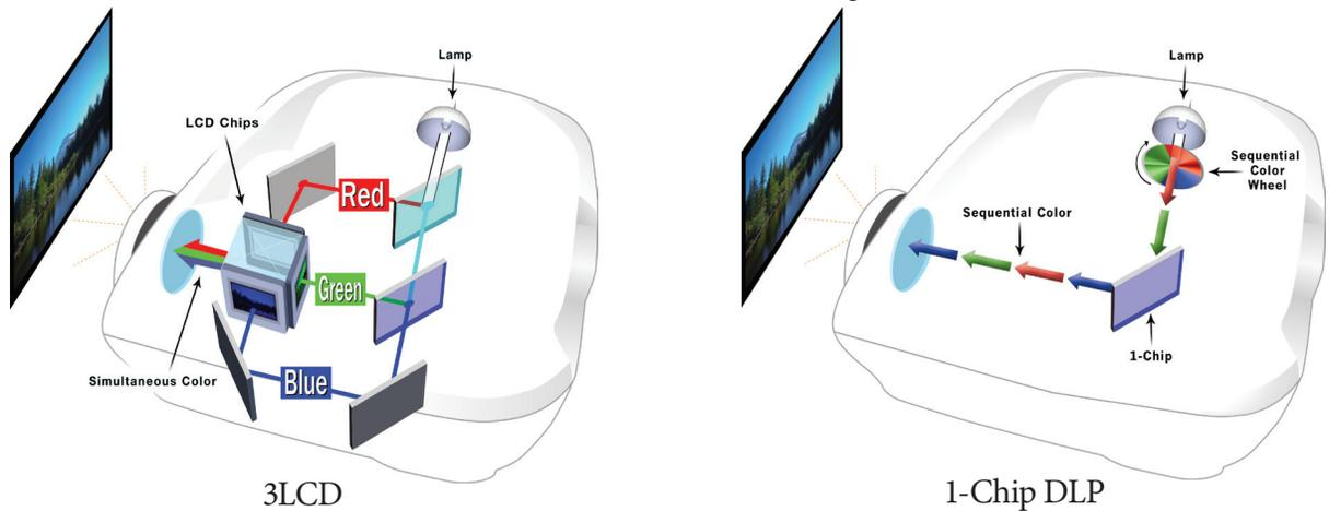
*Figure 2:* There are two types of projector systems used by the majority of the market. Both systems use red, green and blue light, but they work in different ways. 3LCD technology (left) uses 3, LCD chips, while the 1-Chip DLP system uses a rotating wheel of sequential colors (right).
