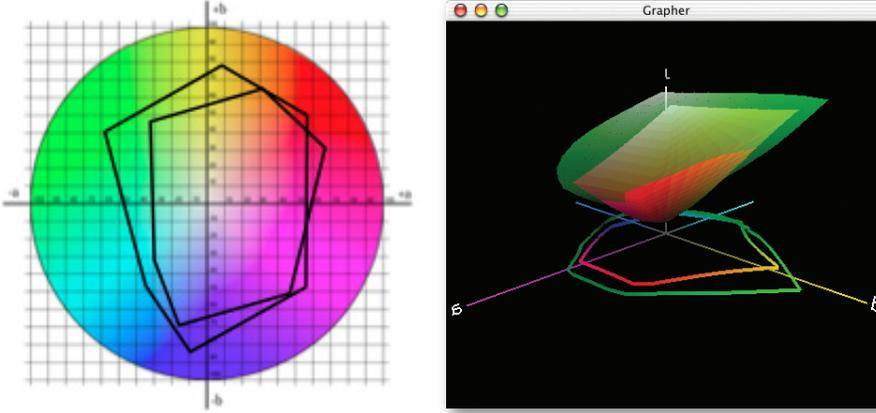
Figure 4: Color diagrams can be shown as 2-dimensional plots (left), but color is really a 3-dimensional phenomenon and we get more information by displaying the color of a projector in a 3-D  $L^*a^*b^*$  plot (right). [From Understanding Color Management, Sharma, Thomson, 2004.]
