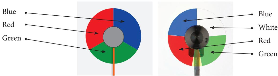
**Figure 6:** 1-Chip DLP projectors do not make a bright white when used in the normal red-green-blue mode (left), so a manufacturer can add a white segment to the sequential color wheel (right), which artificially increases White Light Output, but at the expense of color. Color wheel shown here is from InFocus IN37 1-Chip DLP projector.
