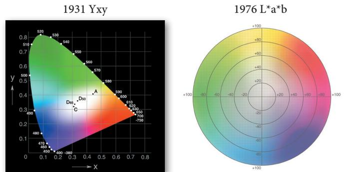
*Figure 3:* The 1931 Yxy diagram (left) is horseshoe shaped and has a large area for green colors but compresses blues and reds. The 1976 L\*a\*b\* diagram (right) affords all colors equal spacing. [From *Understanding Color Management*, Sharma, Thomson, 2004.]
