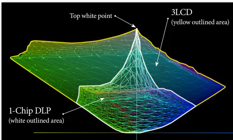
Figure 5: White Light Output also known as White Brightness is measured only at the top white point. Color Light Output also known as Color Brightness makes multiple measurements that include color. Despite their very different color ability, 3LCD and 1-Chip DLP projectors shown here would have the same White Brightness which can lead to making incorrect assumptions about color performance.
