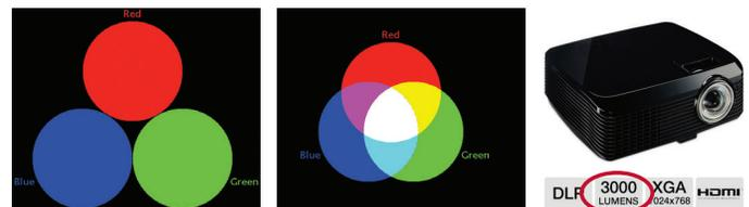
*Figure 1: Projector systems use red, green and blue light to create multiple colors. Where red, green and blue overlap we see this as white. In the past the white has been measured and reported as the “Brightness” level in lumens.*
