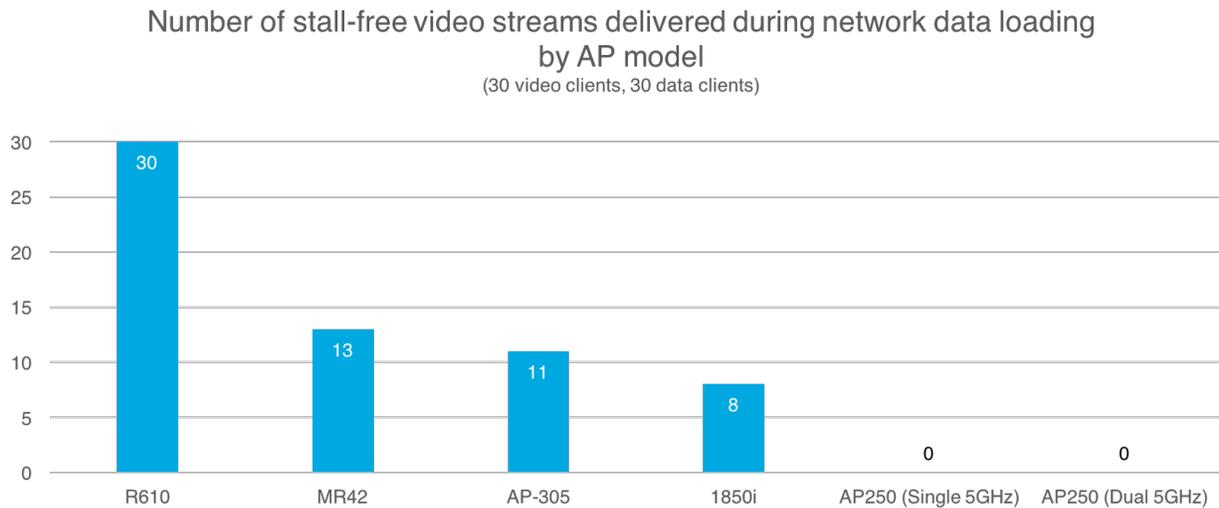
Figure 4 – Test 1 results for stall-free video under load
